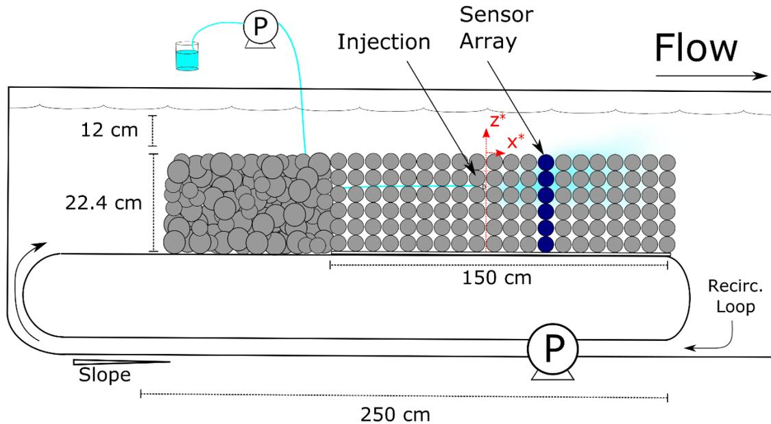
Figure 2.1. Schematic of recirculating flume with bed composed of a flow-condition region of randomly-packed spheres and a test section composed of a cubic-close-packed array of spheres.
