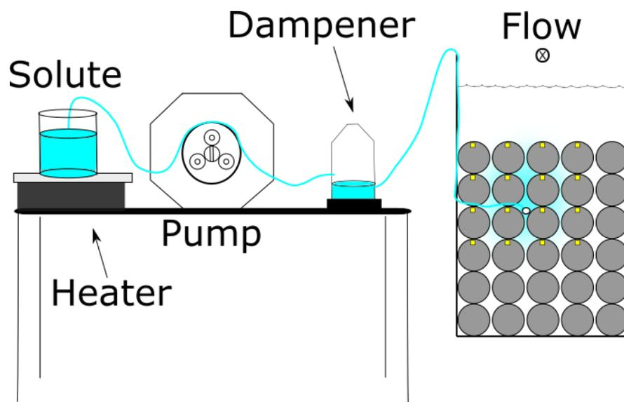
Figure 2.10. Schematic of injection setup. Solute was heated to neutral buoyancy prior to injection. A custom flow dampener (inverted vortex tube with) was installed in-line to minimize pulsation from the peristaltic pump.
