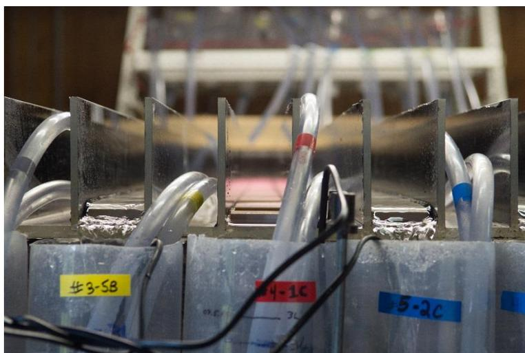
Figure 4.9. Upstream view of flumes from effluent reservoirs. Middle flume (red label) is at the experimental endpoint, with tiles removed for image analysis.
