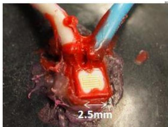
Figure 2.2. Simple-cubic-packed sediment module with sensors installed (left). Sensors were 2.5-mm square interdigitated electrodes fixed to the sediment grains with epoxy and sealed with resistive wax (right).
